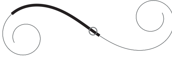
Figure 7.12: An Euler spiral, its inflection point (circle) and a Euler spiral segment (thick black).
